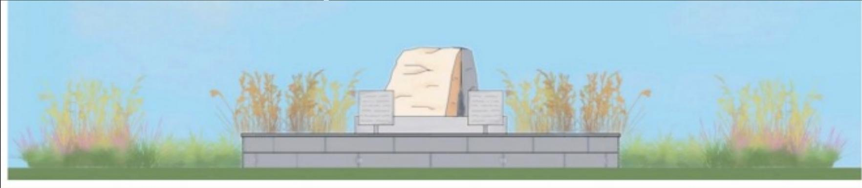
The fountain features two rocks, one granite and the other limestone, representing The Land Between. The 20 ft. retaining wall has a constant 2 in. level of water. The continuous flow of water over the two central rocks completes the fountain. The granite and limestone rocks are 3 ft. high sitting on a round 4 ft. high concrete pedestal.
